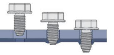
Framo is assembled via thread forming screws. The non-cutting cold formed threads of the screw form their own threads to pilot holes of the perforated Framo profiles. The low thread forming torque and resulting high clamping force, offers a superior process-reliable shake-proof fastening. The thread forming screws are removable and can be used again.
